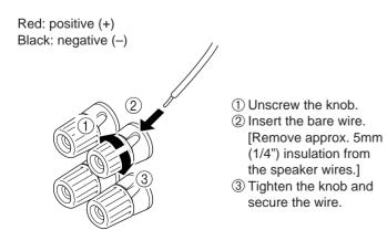
\* Banana Plug connections are also possible (except for Scandinavian model). Simply insert the Banana Plug connector into the corresponding terminal.
